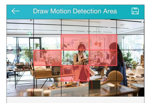
In the selected area, alarm and video recording will occur when the object is detected to move. in the horizontal screen mode, the area selection is more convenient
